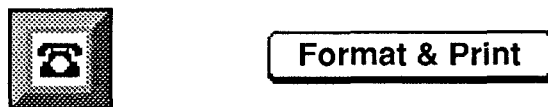
Figure 3. Onscreen buttons seem to protrude from the screen; they afford pushing, but not moving or editing.
